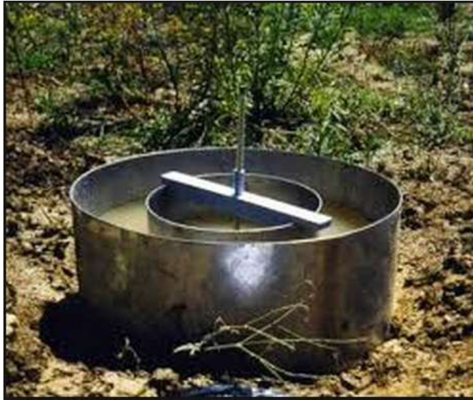
Figure 4.4: Field set up of double ring infiltrometer
